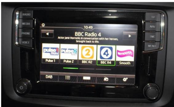
a USB connection for an MP3 player, voice control for some of the features, a menu button to set up many of the features of the car and it can also show pictures from either the USB or SD card. Quite a contrast with the 1950s radio shown on the previous page.
